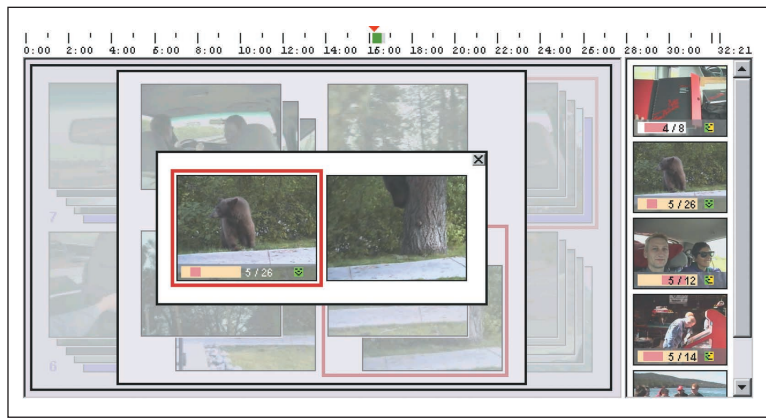
Figure 4. Video editing browser that shows groups of keyframes for a video clip, called piles. The browser sorts the keyframes by color similarity and displays them row by row in the time order of the first clip from each pile. The timeline at the top of the interface shows the coverage of the clips in the pile currently under the mouse cursor, represented by the green area, as well as the start time of the particular clip within that pile, which appears as a red inverted triangle.
